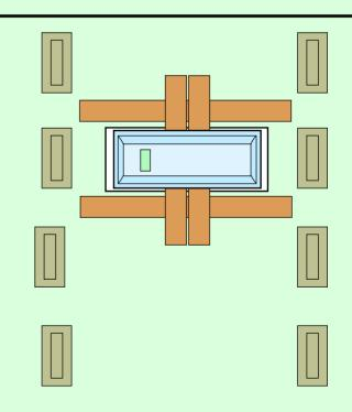
Rotate the burial vault on the M.B.R. TurnTable, and set up an above-ground sealing device to lift the burial vault. Remove the TurnTable & center planks.
