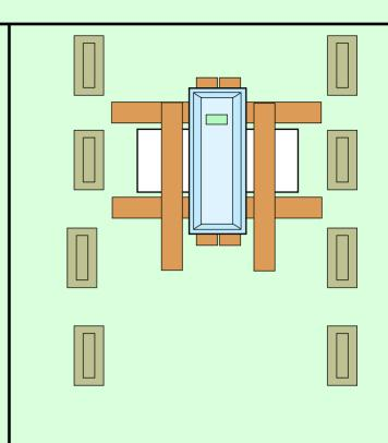
Use M.B.R. Lifterkart to place the burial vault on to the M.B.R. TurnTable.
