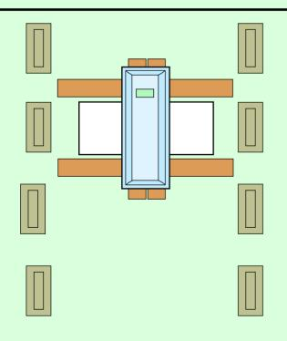
Remove the planks used to drive the M.B.R. Lifterkart over the grave hole.
