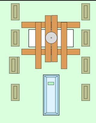
Set up planks around the hole as shown with M.B.R. TurnTable in the center.
